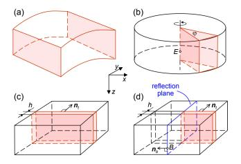
**Figure 3.** Possible symmetries that can be accounted for in the calculation of gravity changes and ground displacement by method A. The simulation domain (red) occupies a region of the subsurface reservoir (black).
