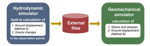
Figure 2. Diagram showing the software options for modelling gravity changes and ground displacement. The interface between the simulators is organised through external files.
